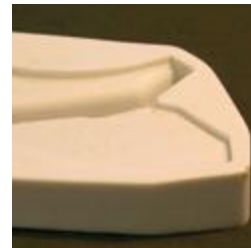
Ceramacast™ 900-N casts small, dense part.
