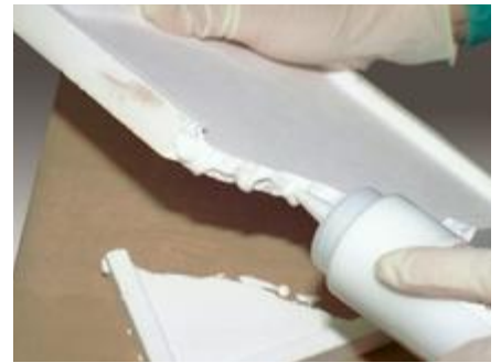
Cerabond™ 503 repairs furnace saggar plate.
