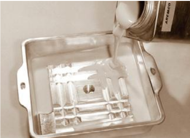
Place the machined master, a duplicate of the finished casting, into a pan, and pour the EZ-Cast™ over the master.
