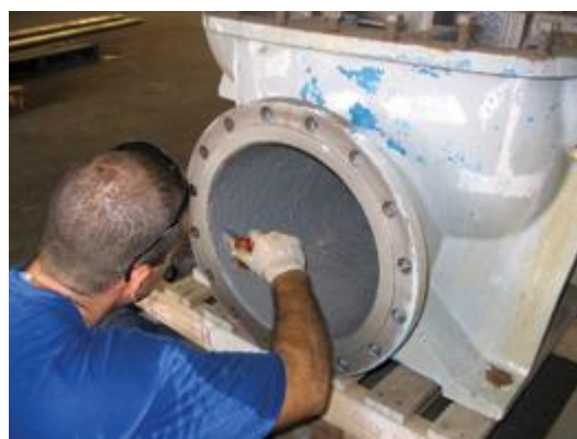
Corr-Paint™ CP2060 coats pump housing.
