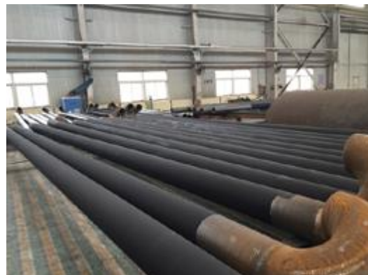
HiE-Coat™ 840-M coats gas-fired heating tubes.
